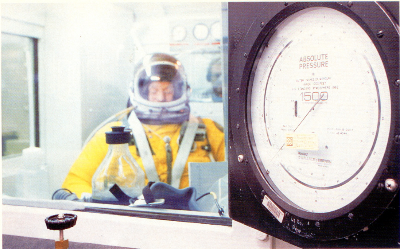
After decompression to 73,000 feet in the altitude chamber, the author's spacesuit is fully inflated (above). Note the beaker of boiling water in the chamber (above). Wearing virtual-reality goggles, the author steers a parachute landing (top left). Practice is required to exit a U-2 gracefully while wearing a spacesuit (above left).
